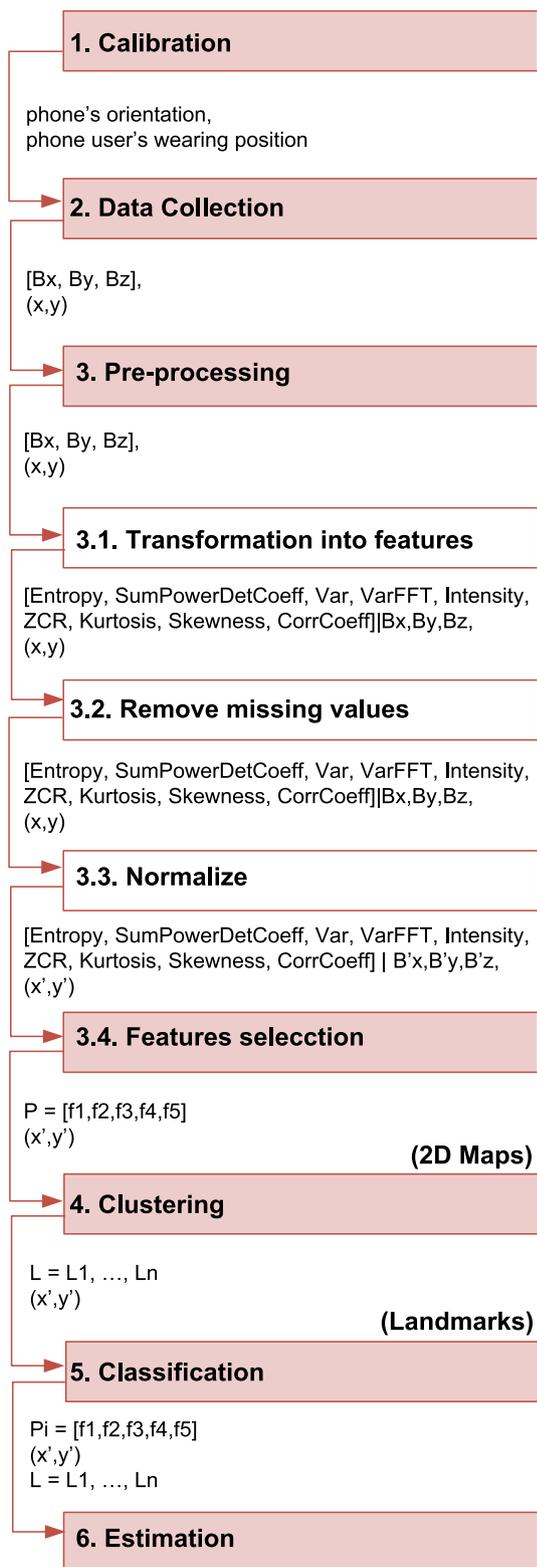
**Fig. 1** Off-line phase of the localization mechanism
