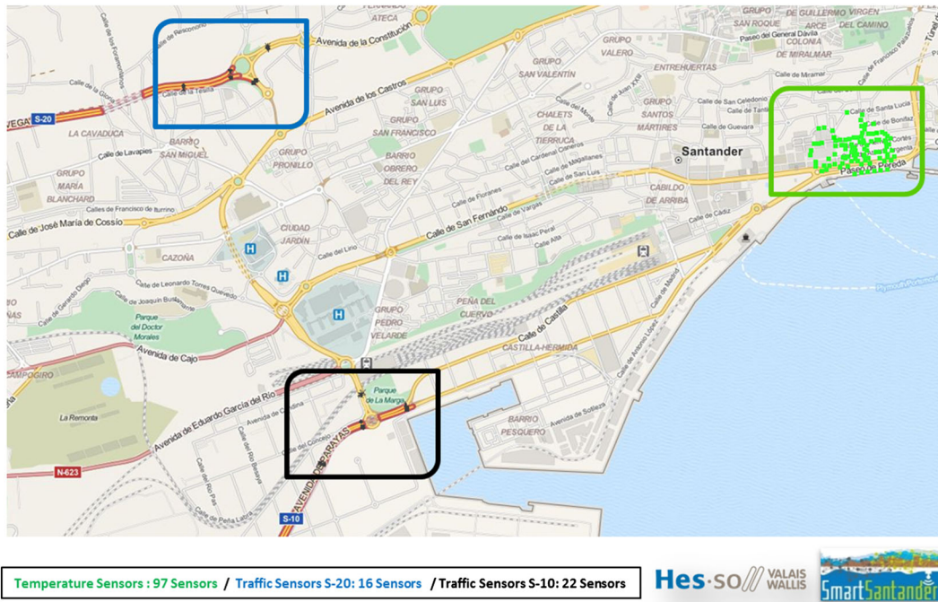
Figure 1. SmartSantander testBed (traffic and temperature deployment).
