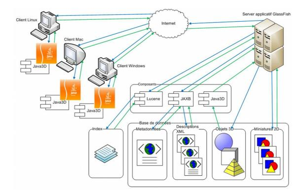
Figure 3: Global architecture of the developed application including the various base data and application used to provide the functionality for textual and visual retrieval using a web interface.
