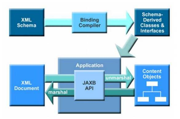
Figure 2: Mechanisms of JAXB to convert between XML and Java objects and vice versa.
