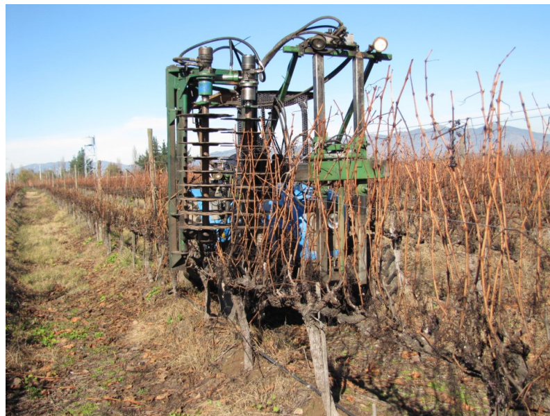
Figure 1. Prepruning machine of a Royat vineyard.
