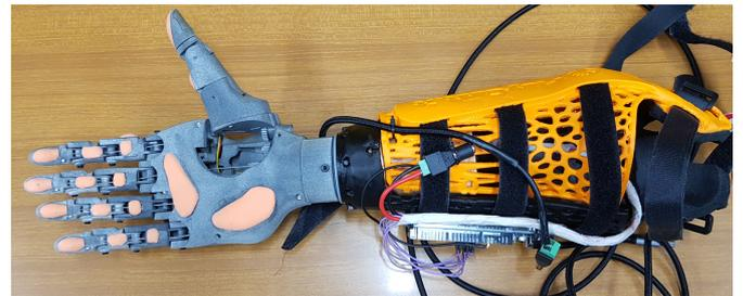
Fig. 1: 3D printed robotic hand and socket.
