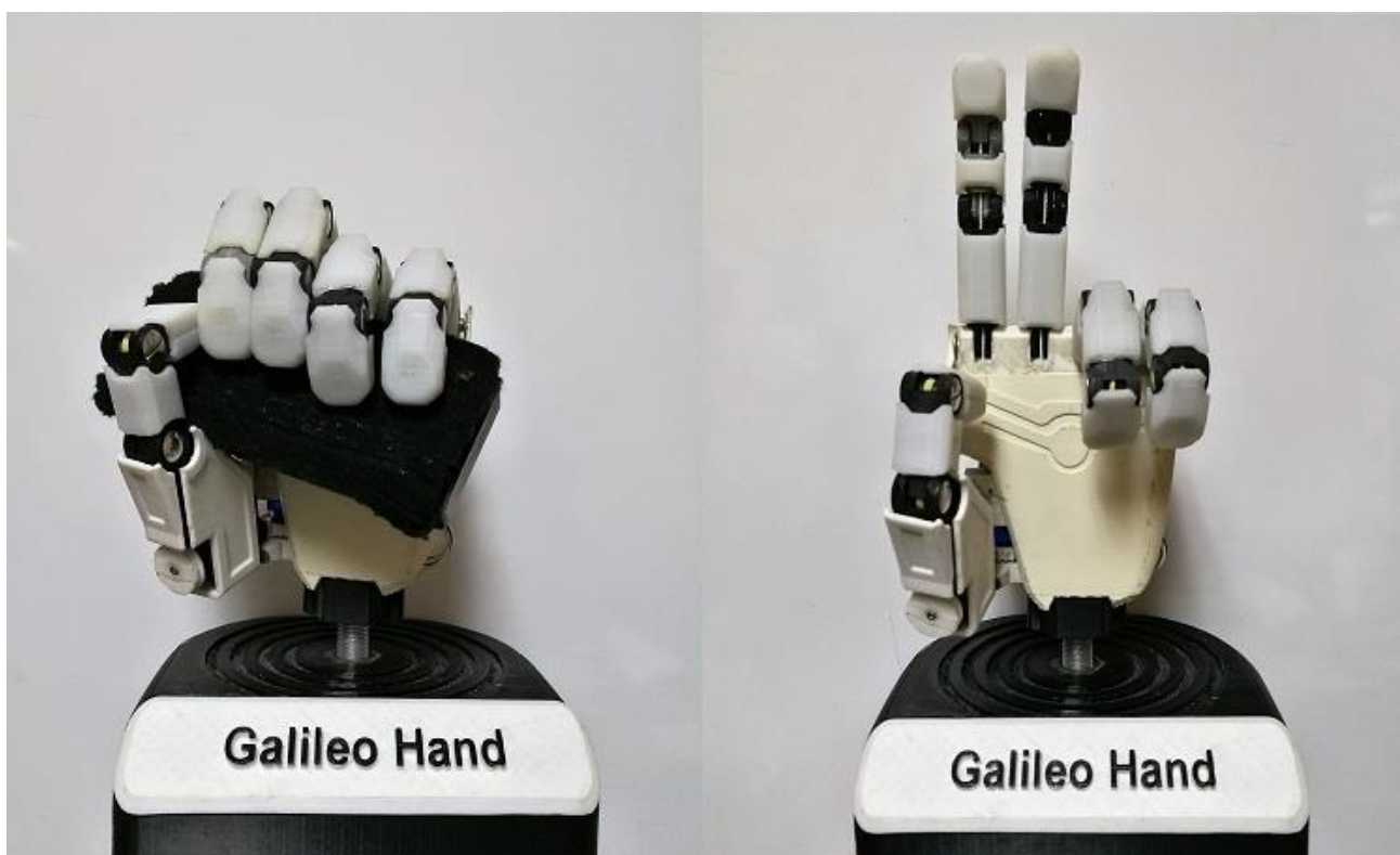
Figure 12. Galileo Hand performing power grasping and peace sign 55 .
