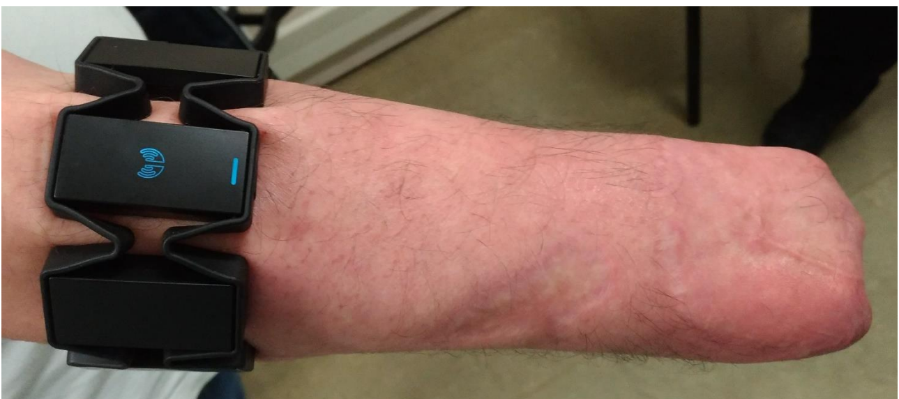
Figure 4. Myo bracelet on a stump 21,22 .
