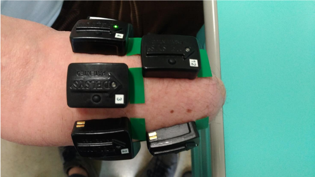
Figure 5. sEMG electrodes placed on a stump 21,22 .
