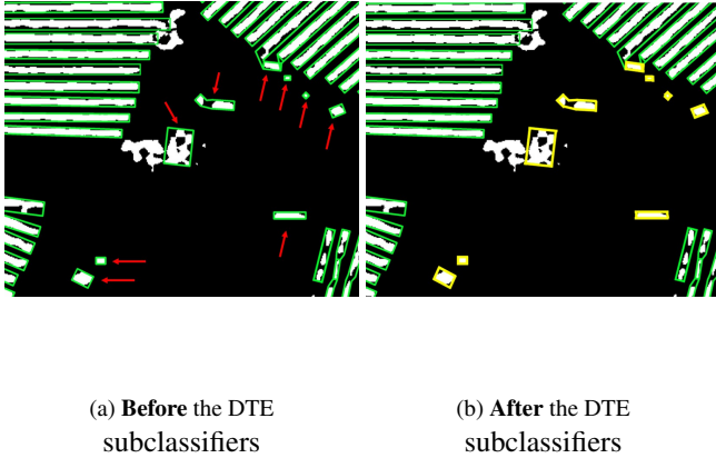
Fig. 6: Visualization of the classification results for lines of vines with the altered U-Net. Image (a) represents the classification at the output of the U-Net, by applying an edge algorithm. Image (b) represents the output of the U-Net after filtering using a DTE on the detected areas. The green are the rectangles detected as vine lines. The red arrows show false positives. The yellow are the rectangles with a corrected classification after the DTE.
