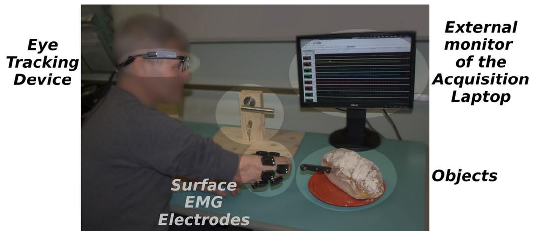
**Fig. 1** Overall view of the acquisition setup.
