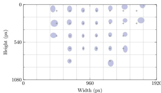
**Fig. 2** The accuracy and precision of the eye tracking with respect to the location within the video frame. For each patch, the shift of the ellipse center with respect to the cross indicates the accuracy in either axis of the gaze within that patch. The radii of the ellipse on the other hand indicate the precision.
