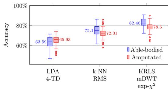
**Fig. 6** Classification accuracies for able-bodied and amputated subjects when predicting the grasp type with three different types of classifiers.
