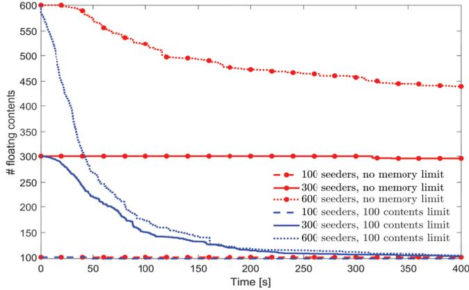
Fig. 4: Mean number of floating contents over time in a localized floating system, for different initial number of seeders. Node speed is equal to 10 m/s, and node density is  $800 \text{ users}/\text{km}^2$ .
