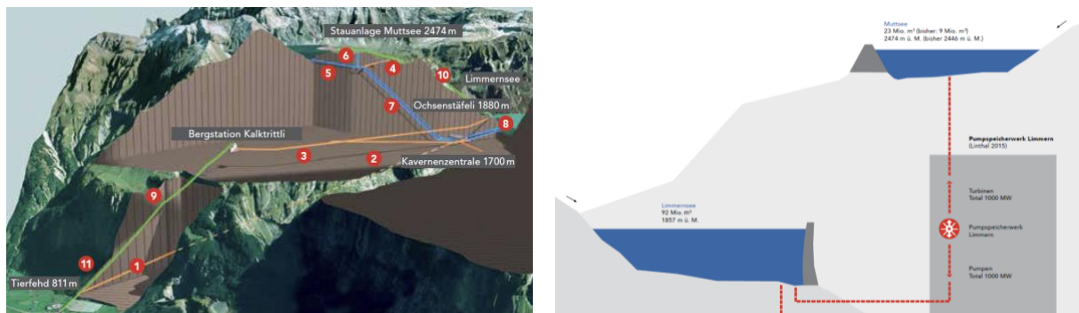
Figure 1. Cutaway graphics of the Limmern PSHP (source:[13]).
