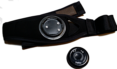
Figure 1: The Zephyr BioHarness 3 used for the data acquisition phase for the D1NAMO dataset [7].
