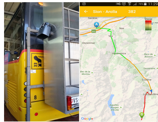
Fig. 2. Road surface sensor installation (left) and RSM interface (right).
