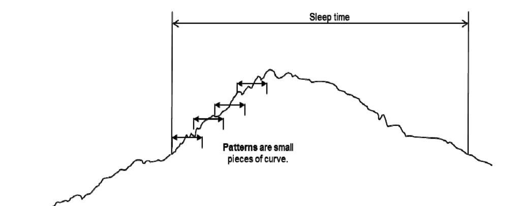
The figure shows a schematic example of Triggerfish curve (−). We consider pieces of curves as potential patterns (↔). All the pieces have the same length and may overlap adjacent pieces. The length of the pieces and the length of overlapping are two tuning parameters when searching for patterns in curves.
