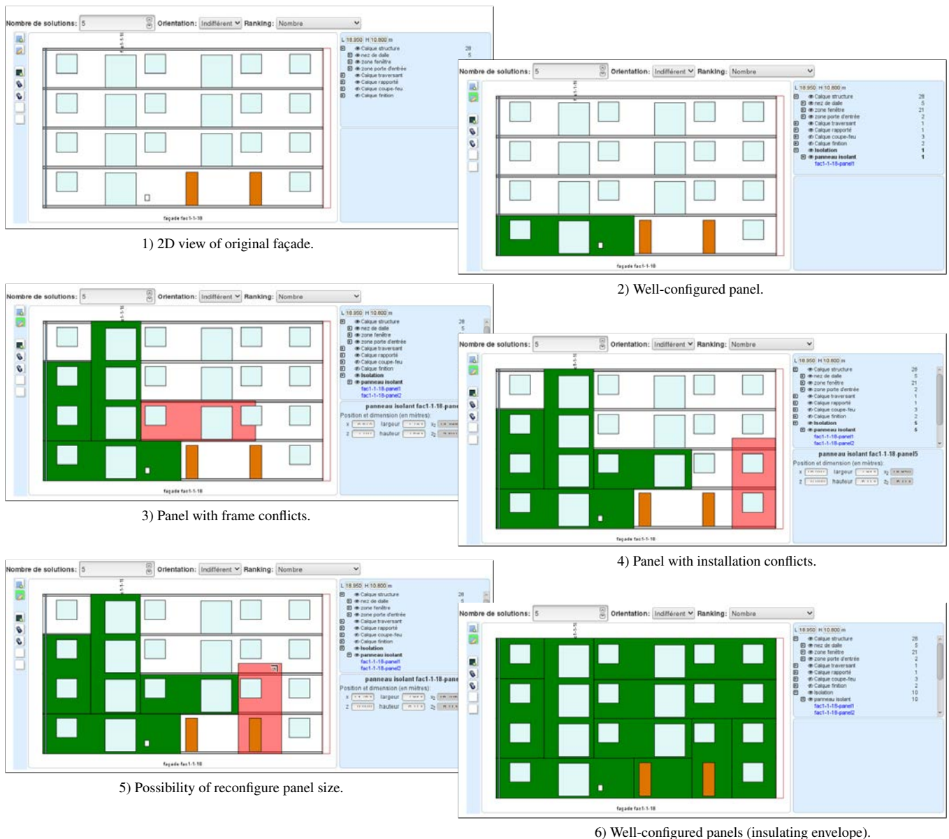
Figure 2. Demonstration: System actions through normal execution.
