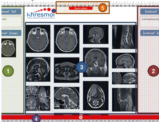
Fig. 3. User interface of Shambala. Zone (1) is for 'drag-and-drop' of images relevant for search and for keyword input. Zone (2) is for irrelevant images and keywords. Zone (3) is provides a results view. Zone (4) allows for uploading images. Zone (5) allows the configuration of search options.
