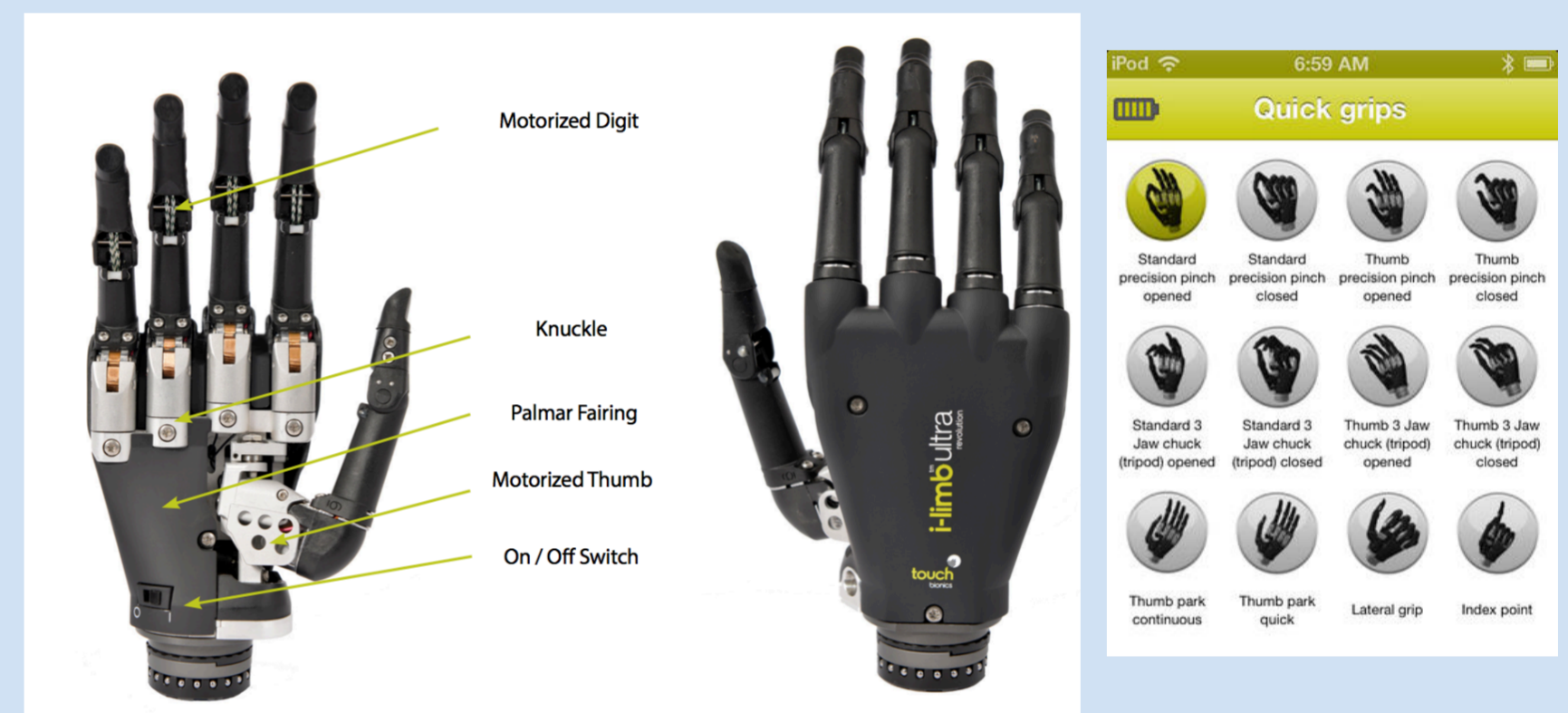
Figure 1: Example of a modern prosthesis with high mechanical functionalities. The Touch-Bionics i-limb ultra
